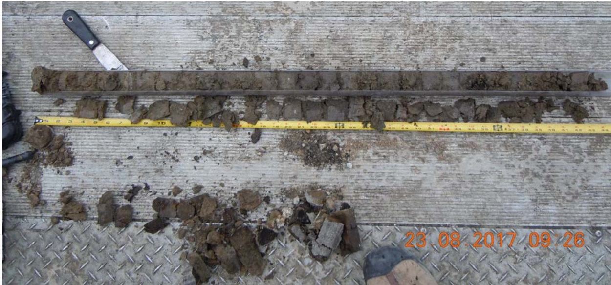
Figure 5: Split-Spoon Core Sample (BH20 – Core 2)
